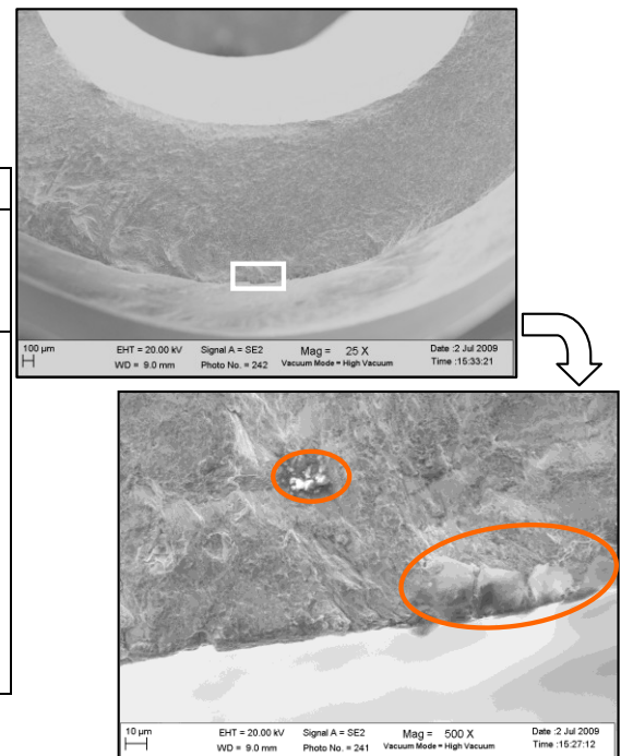
Fig.7. Fatigue crack origin exhibiting high Mo concentrations in the encircled region
